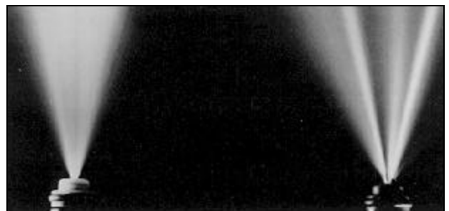
Clean Injector Spray Pattern
