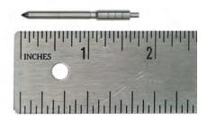
Fuel injectors in high-pressure common-rail diesel engines use smaller, highly engineered components to produce the higher fuel pressures needed for improved combustion. The tighter clearances invite internal diesel injector deposits that interfere with injector needle actuation, reducing performance. External deposits can also form on the injector
