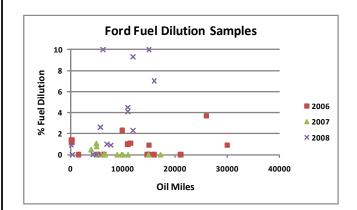
As illustrated in the charts, model-year 2007 and newer light-duty diesels are experiencing higher fuel dilution than previous model years. Although these vehicles are experiencing higher fuel dilution, regeneration cycles vary based on service (engines operating in severe service conditions do not actively regenerate as often as engines operating in
