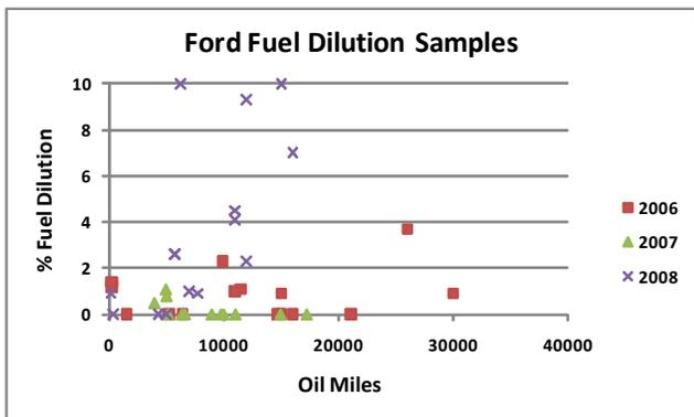
As illustrated in the charts, model-year 2007 and newer light-duty diesels are experiencing higher fuel dilution than previous model years. Although these vehicles are experiencing higher fuel dilution, regeneration cycles vary based on service (engines operating in severe service conditions do not actively regenerate as often as engines operating in
